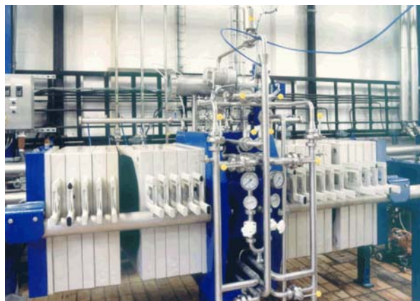
Fig. 2 : pilot thinbed membrane filter
