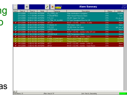
SCADA Alarm Summary screen (showing collect prompts)
