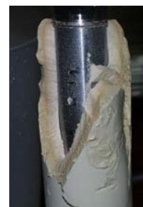
Figure 7: Filter candle coated with Crosspure®
